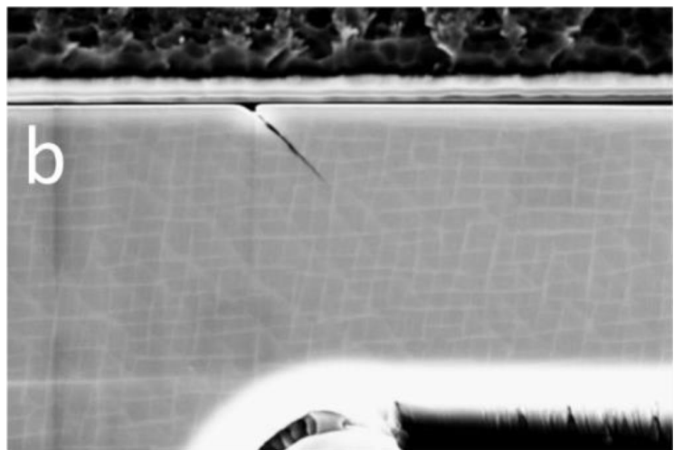
Fig 4: Micro-bending beam with an artificial fatigue crack (the beam thickness is 10 μm).
