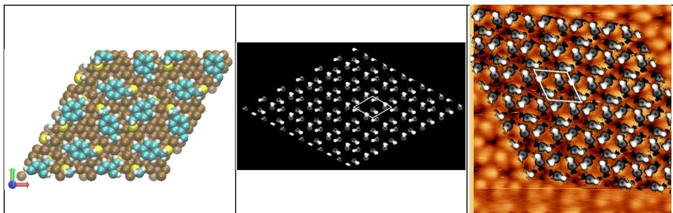
Fig. 3: Left panel: molecular arrangement obtained by DFT calculations with Ag vacancies on the top most layer. Center panel: simulation of the corresponding STM image. Right panel; comparison between the experimental and calculated 10x10 nm<sup>2</sup> STM images.
