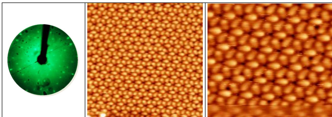
Fig.2: Left panel: LEED pattern for the low coverage lying down phase of BDMT on Ag (111). Center and right panels: STM images of the corresponding molecular arrangement in 20x20 nm<sup>2</sup> and 10x10 nm<sup>2</sup> areas, respectively.
