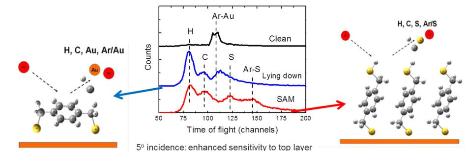
Fig.1: Schematics of molecule orientation. Left: lying down phase, Center: corresponding ion scattering spectra, Right: standing up phase.
